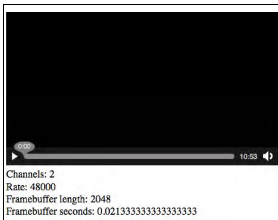
Figure 8–3. Getting information about the audio sample values in the framebuffer
