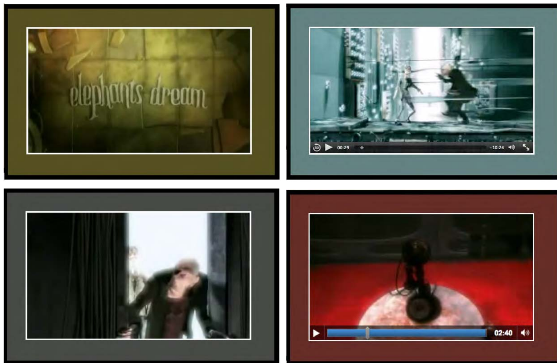
Figure 6–9. Rendering of an ambient CSS color frame in Firefox (top left), Safari (top right), Opera (bottom left), and Google Chrome (bottom right)
