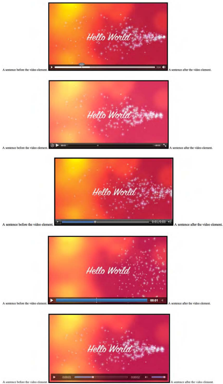
Figure 3–2. A <video> inline in Firefox, Safari, Opera, Chrome, and IE (top to bottom)
