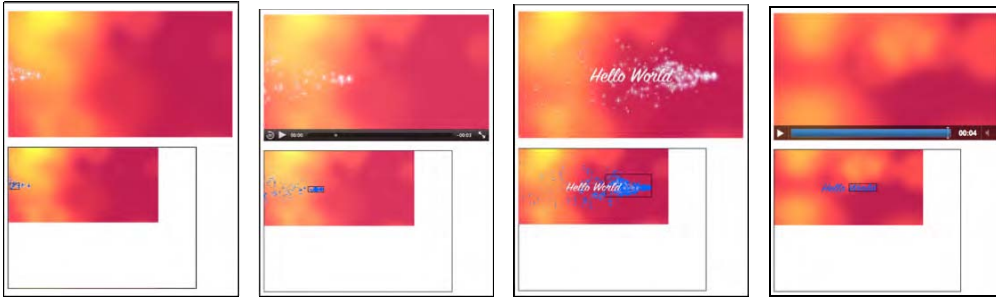
Figure 7-5. Image segmentation results on a motion detected video in Firefox, Safari, Opera, and Chrome (left to right)
