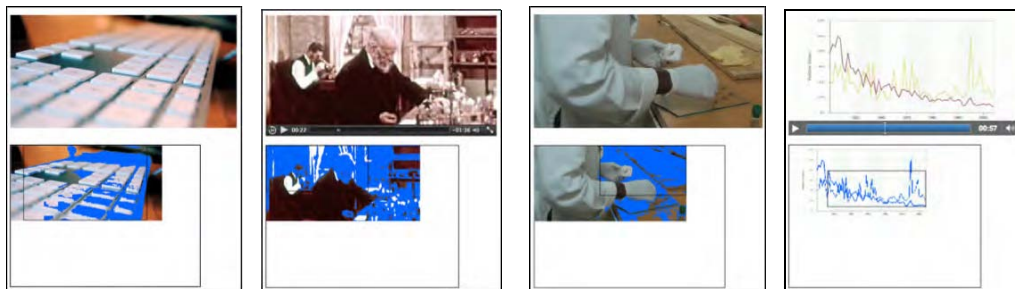
Figure 7-7. False positives on face detection using skin color in Firefox, Safari, Opera, and Chrome (left to right).
