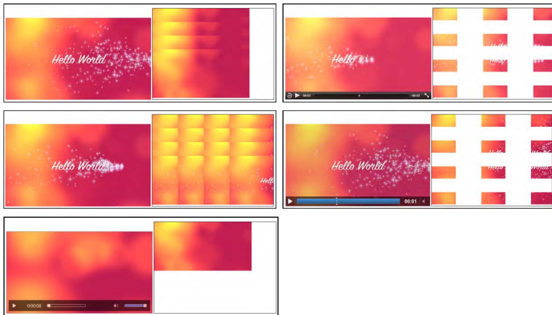
Figure 6–5. Attempted tiling of a video into a Canvas using putImageData() in Firefox, Safari (top row), Opera, Chrome (middle row), and IE (bottom)
