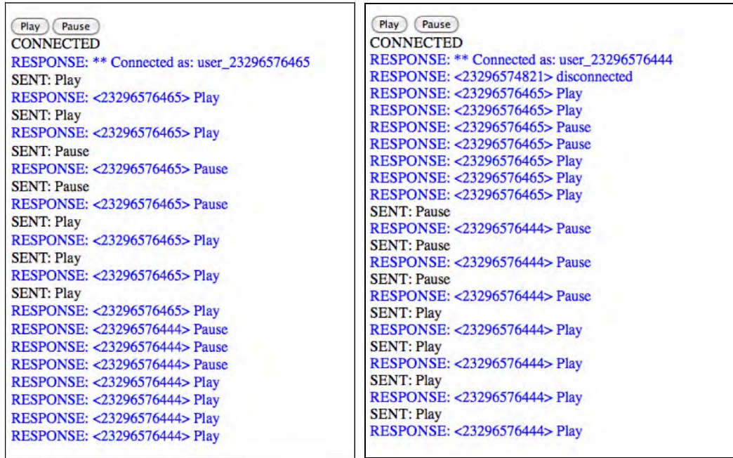
Figure 10–4. WebSocket example of communicating sides, left in Firefox, right in Google Chrome
